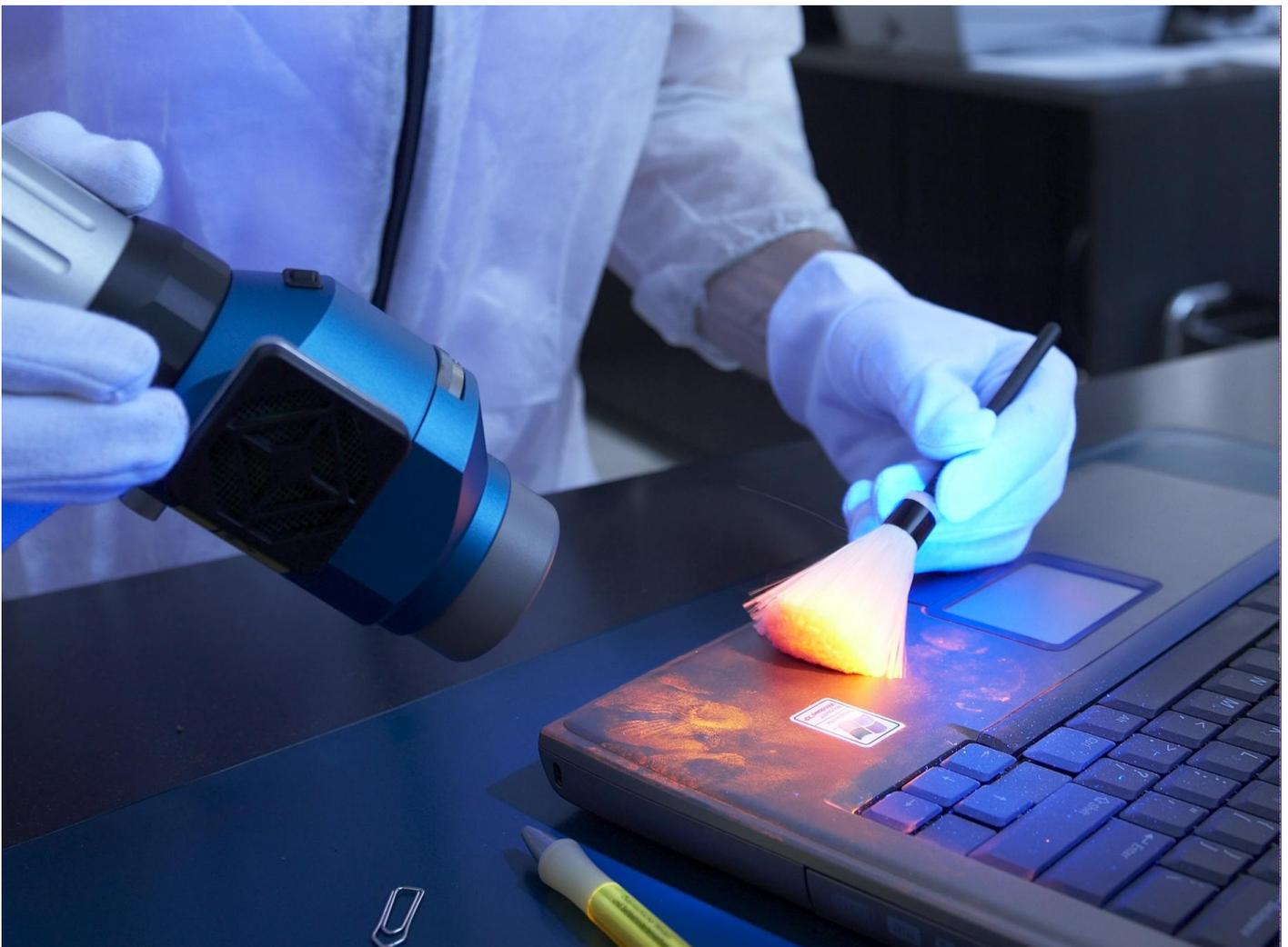
The SL-450 is fully portable. No interconnected cables or shoulder packs. Therefore unlimited movement around the crime scene is guaranteed. The Xenon powered light source submits an outstanding light output for general crime scene investigation. Seven different spectra from UV 365 nm, white light up to 530 nm are built-in.
