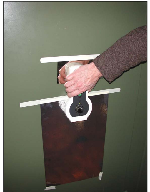
Lifting a dust print from a vertical surface
