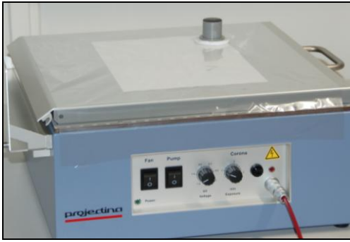
New toner pad technique for cleaner image development maintaining excellent sensitivity - avoids constantly recovering of cascade beds
