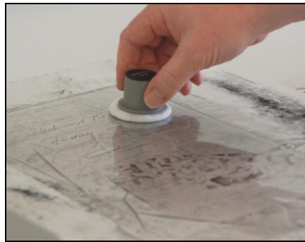
New toner pad technique for cleaner image development maintaining excellent sensitivity - avoids constantly recovering of cascade beds
