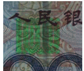
IR 740-1100 NM ILLUMINATION FOR "ANTI-STOKES INKS" EXAMINATION
