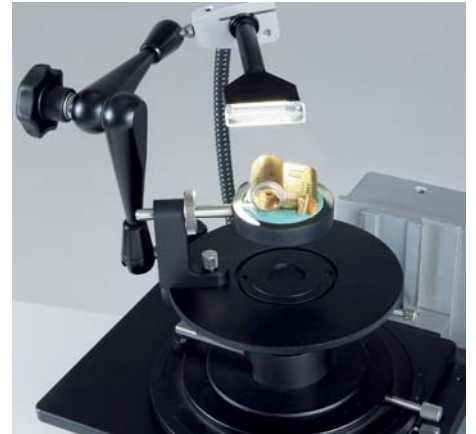
Tool mark stage with plasticine holder
