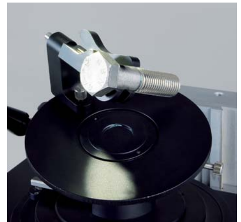
Tool mark stage with grip holder
