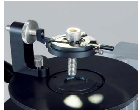
Tool mark stage with three-point fixing clamp
