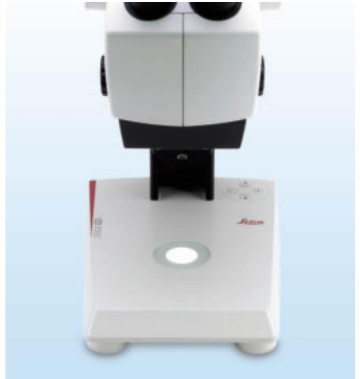
4. Transmitted light for transparent and semi-transparent samples
