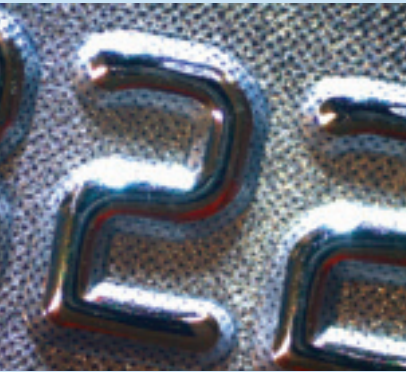
Steep incident light with the 3 upper diodes
